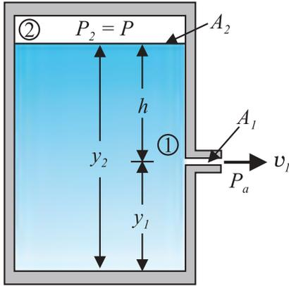
**Fig. 9.10** Torricelli's law. The speed of efflux,  $v_1$ , from the side of the container is given by the application of Bernoulli's equation. If the container is open at the top to the atmosphere then  $v_1 = \sqrt{2gh}$ .
