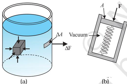
**Fig. 9.1** (a) The force exerted by the liquid in the beaker on the submerged object or on the walls is normal (perpendicular) to the surface at all points.
