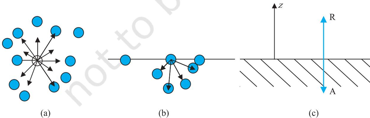
**Fig. 9.14** Schematic picture of molecules in a liquid, at the surface and balance of forces. (a) Molecule inside a liquid. Forces on a molecule due to others are shown. Direction of arrows indicates attraction of repulsion. (b) Same, for a molecule at a surface. (c) Balance of attractive (A) and repulsive (R) forces.
