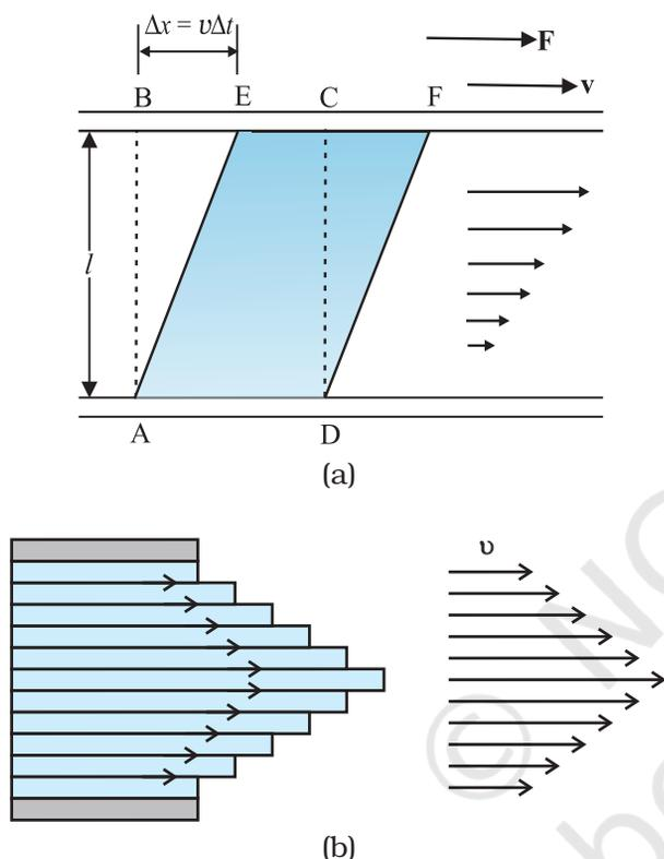
**Fig 9.12** (a) A layer of liquid sandwiched between two parallel glass plates, in which the lower plate is fixed and the upper one is moving to the right with velocity  $v$
