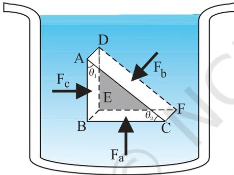
**Fig. 9.2** Proof of Pascal's law. ABC-DEF is an element of the interior of a fluid at rest. This element is in the form of a right-angled prism. The element is small so that the effect of gravity can be ignored, but it has been enlarged for the sake of clarity.
