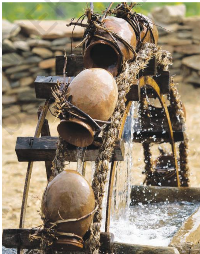
Fig. 2.29. A Persian wheel used to draw water from wells or tanks to irrigate fields.
