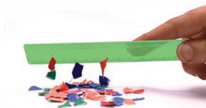
Fig. 5.8: Charged plastic scale attracting small paper pieces
