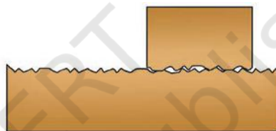
Fig. 5.6: Friction between two surfaces due to irregularities
