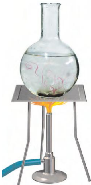
Fig. 3.9 Convection of heat in water
