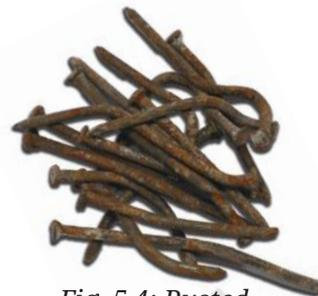
Fig. 5.4: Rusted iron nails
