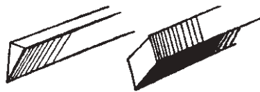
Pointed burin for copper engraving
