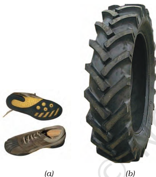
Fig. 9.11 : (a) Soles of shoes and (b) tyres are treaded to increase friction.
