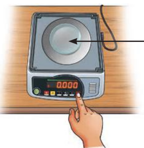
Fig. 9.12(b): Tare the balance after placing a watch glass
