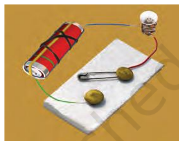
Fig. 9.9 An electric circuit with a switch
